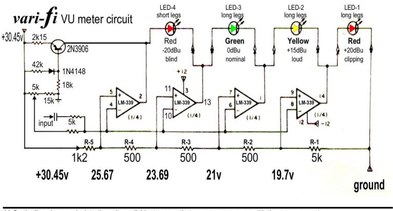
1.) On the line above, calculate the voltage divider to prove that your answers agree with the measurements.
