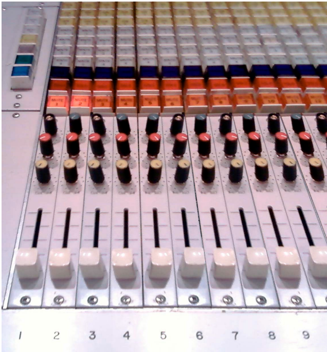
FIGURE-2: The Tape Monitor section, called the "Juke Box," from an API console. The knobs are for Cue (2, prefader) and FX (1, post fader)
